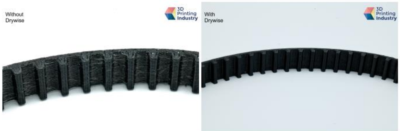
Drive belt 3D printed with non-dried and dried filament. Photos by 3D Printing Industry.
