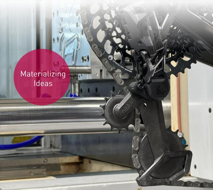
The shifting precision and speed of derailleurs depend directly on the rigidity of the derailleur cage. Therefore, a material based on extended carbon fiber technology (LUVOCOM XCF compound) was selected. This material combines maximum stiffness and strength with exceptionally high impact energy absorption - important characteristics for an MTB pulley cage of this performance class.
