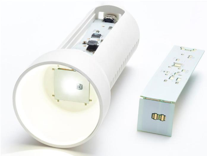
Flashlight with high-performance LED and integrated circuit board
