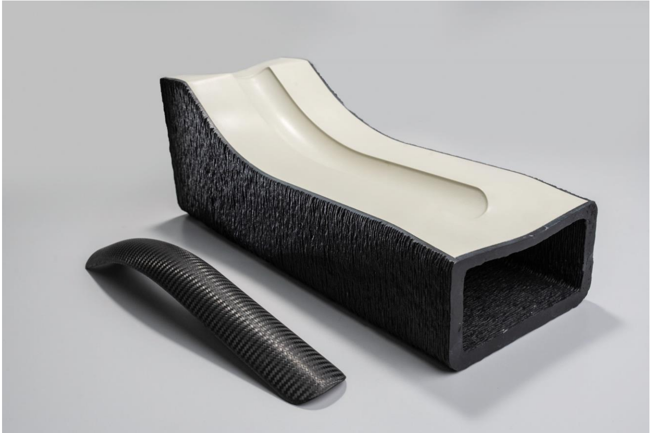
Photo: Usable mold with coated cavity. In the foreground, molded CFRP component
