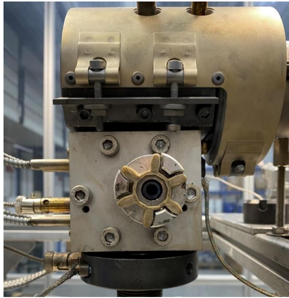
Fig. 3: 3D-printed gear made of LUVOCOM 3F PEEK
