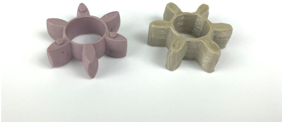
Fig. 1: Gear made of PUR and 3D-printed gear made of LUVOCOM 3F PEEK 9581 NT
