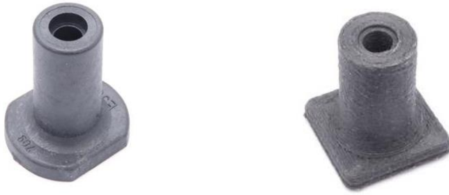
Fig. 4: left: injection-moulded screw boss; right: printed screw boss
