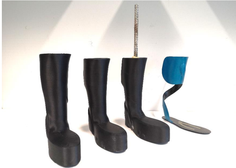
Figure 5. 3D printed mold, mold with handle, final CFRP orthotic
